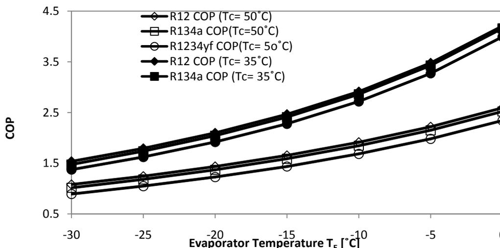
Fig. 3.3 Variation in COP with evaporator temperature
