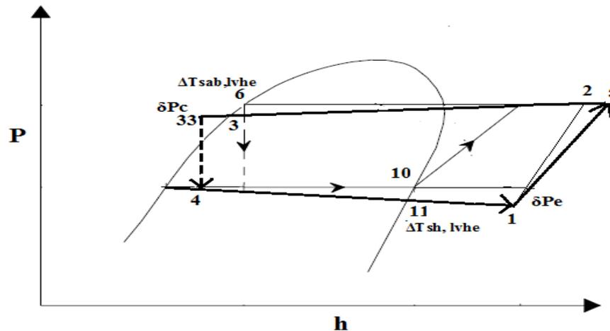
Fig. 2.2 p-h diagram showing subcooling and superheating
