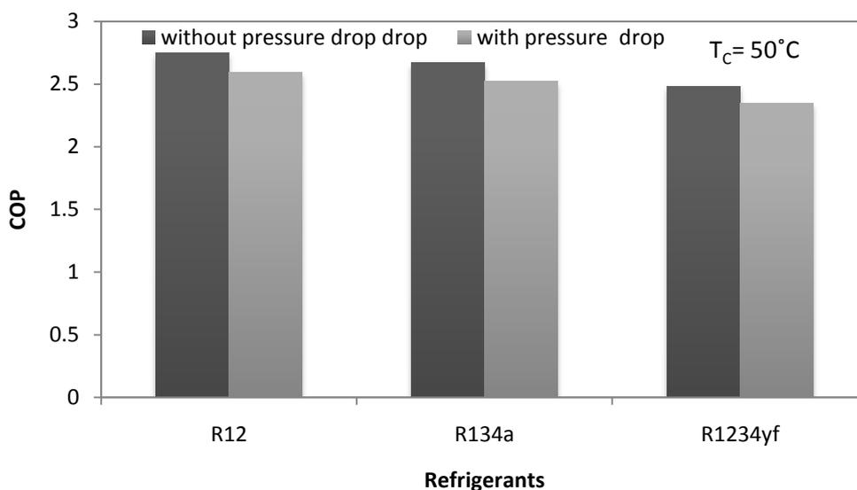
Fig. 3.6 shows variation in COP with and without pressure drop in the evaporator and condenser at  $T_C = 50^\circ\text{C}$ .
