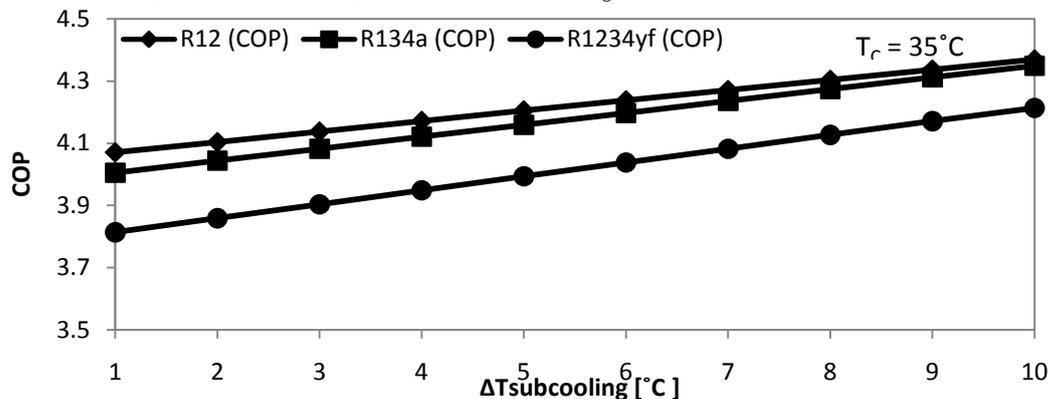
Fig.3.4 Variation in values of COP of system with degree of subcooling
