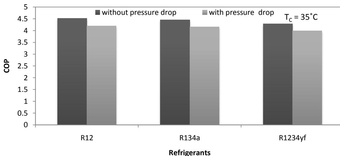
Fig. 3.7 shows variation in COP with and without pressure drop in the evaporator and condenser at  $T_C = 35^\circ\text{C}$ .
