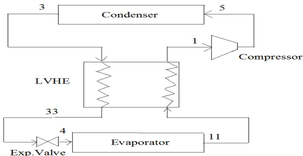
**Fig. 2.1** Schematic diagram of actual vapour compression system with liquid vapour heat exchanger
