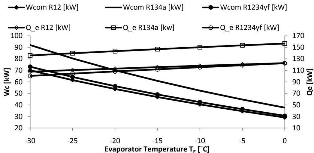
Fig.3.1 Variation of compressor work & refrigerating effect with evaporator temperature
