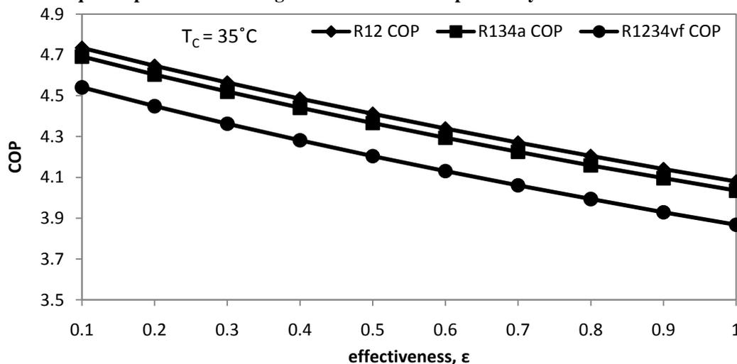
Fig. 3.5 Variation in value of COP of system with effectiveness of liquid vapour heat exchanger
