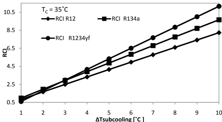
Fig. 3.3 Variation in RCI with degree of subcooling
