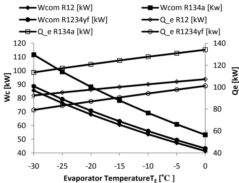
Fig 3.2 compressor work & refrigerating effect with evaporator temperature
